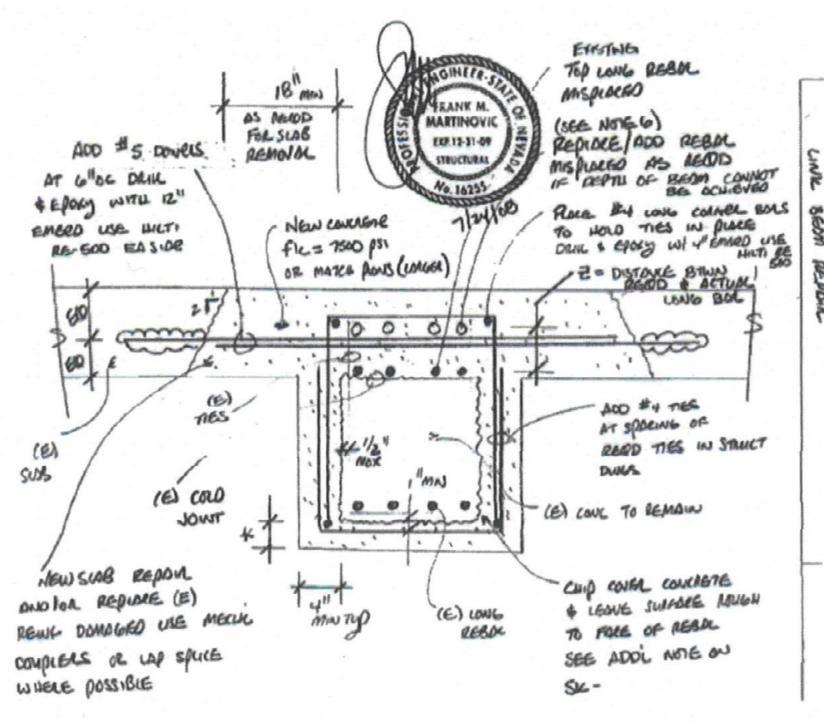
Typical Link Beam Repair Sketch, Plan
